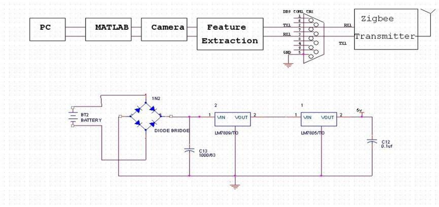
Fig 2.2.1: Schematic diagram of transmitter section
