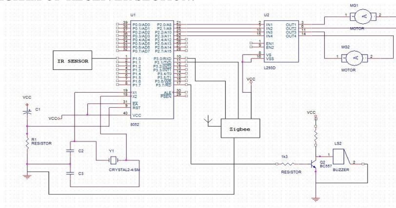
Fig 2.2.2: Schematic diagram of receiver section
