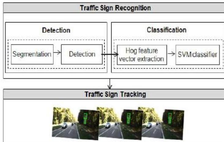
Fig 3.1.4: The proposed traffic sign recognition and tracking process.
