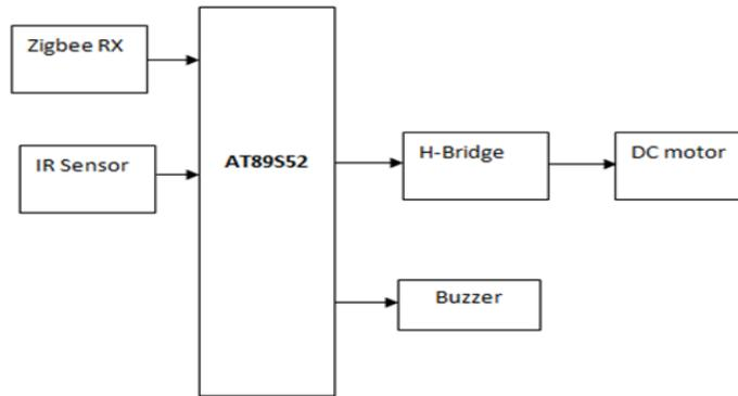
Fig 2.1.2: Block diagram of receiver section
