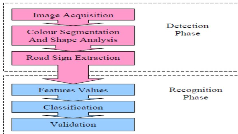
**Fig:3.1.1 Block diagram of the road sign recognition and classification.**
