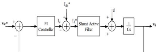
Fig. 5 Control scheme of  $V_c$
