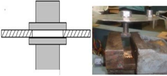
Fig. 2.a. Natural frequencies are detected by hitting the plates
