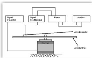
Fig. 3 Experimental set up
