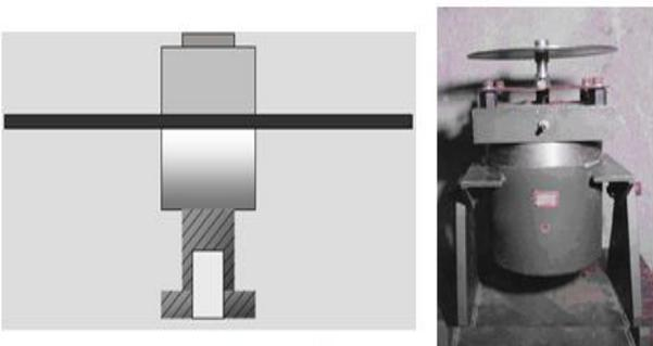
Fig. 2.b. Natural frequencies are detected by using exciter
