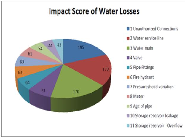
Figure 2: Showing impact value of each type of water loss occurrence in water distribution system.
