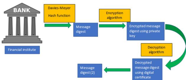
Figure 10: Phase-2 Identity proof & integrity checking
