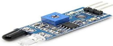
Fig:6 IR sensor with IR transmitting & Receiving LED
