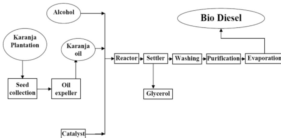
Fig.3 Preparation of laboratory samples of esterified karanja oil (bio diesel)
