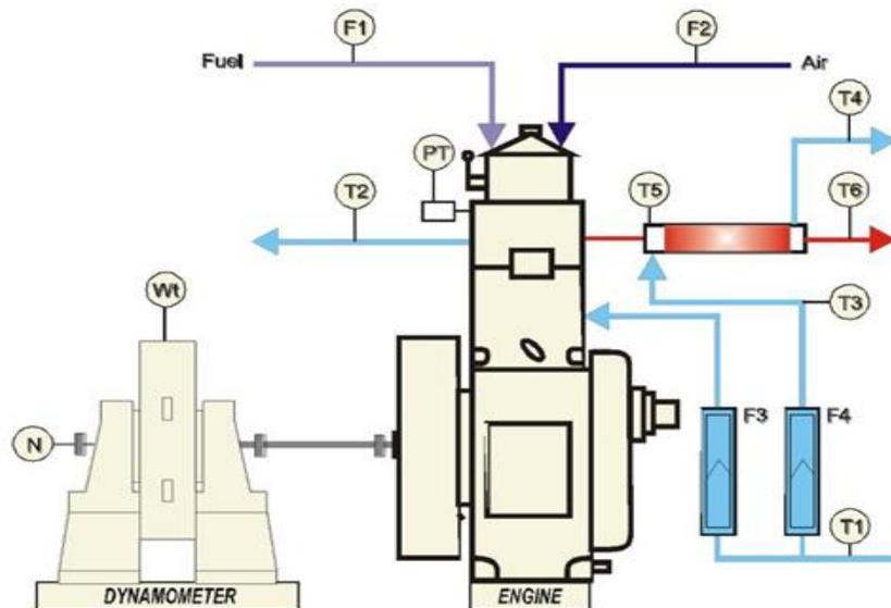
Fig.4 Schematic arraignment
