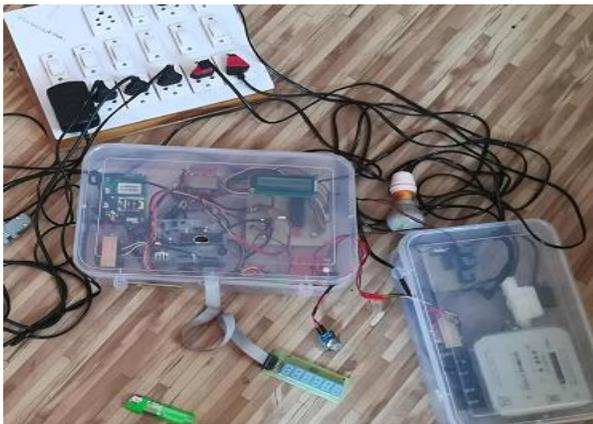
Fig.2 LPG detection and Prevention Unit
