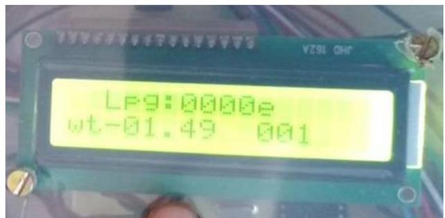
Fig.10 Weight is below threshold shown by LCD
