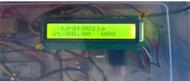
Fig.6 LPG Detection on LCD
