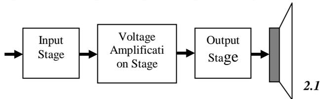
Figure 2. Practical audio power amplifier stages
