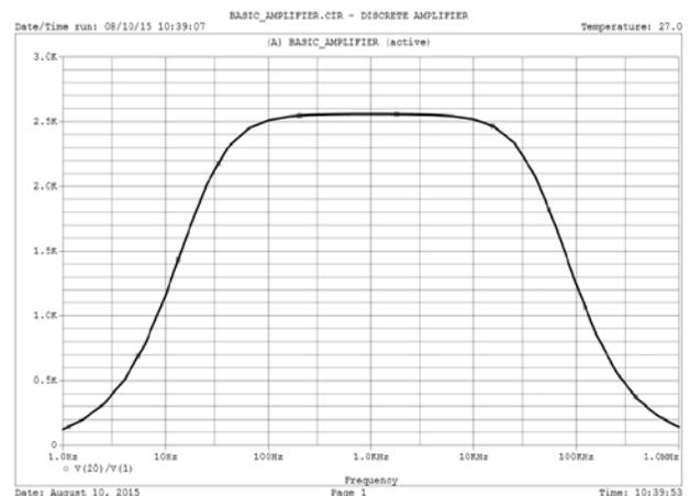
Figure 6 Simulated open loop gain  $A_{ol}$  of proposed amplifier
