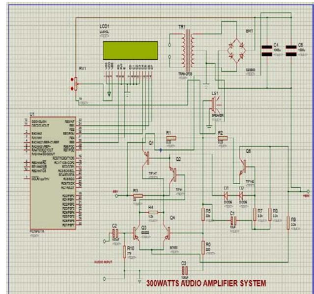
Figure 4. Model of audio amplifier including the LCD
