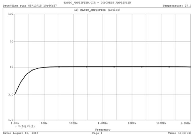
Figure 7. Closed loop gain  $A_{cl}$  of the proposed amplifier
