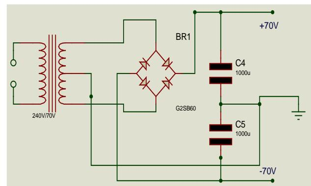
Figure 3. Dual voltage power supply
