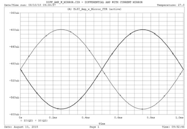
Figure 9. Signal balance of transistors  $Q_1$  and  $Q_2$  at the differential input stage.
