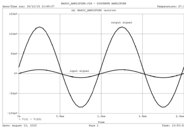
Figure 8. Circuit in operation as an amplifier
