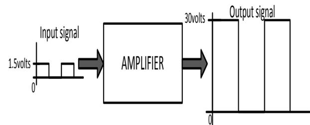
Figure 1. Diagram showing operation of an amplifier
