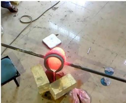
Figure.7. Pouring of molten metal into mold
