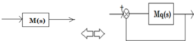
Figure 2. Equivalent closed loop of open loop system
