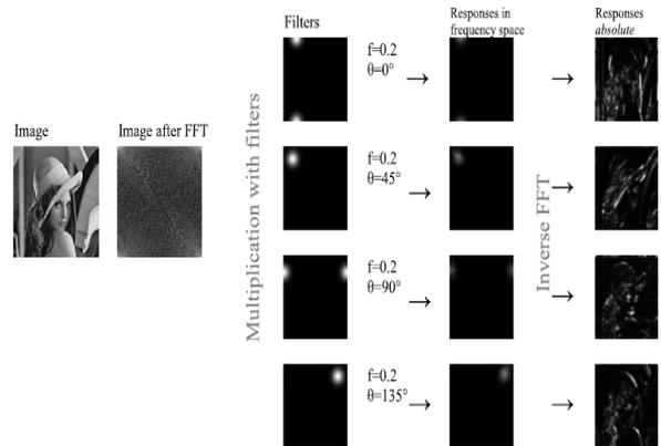
Figure 2. Frequency domain filtering
