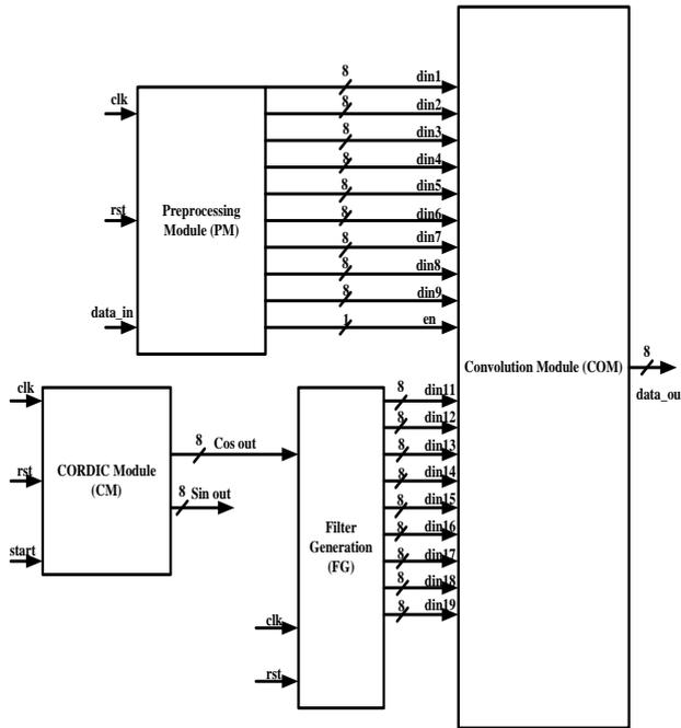
Figure 4. Internal Design of Gabor Filter
