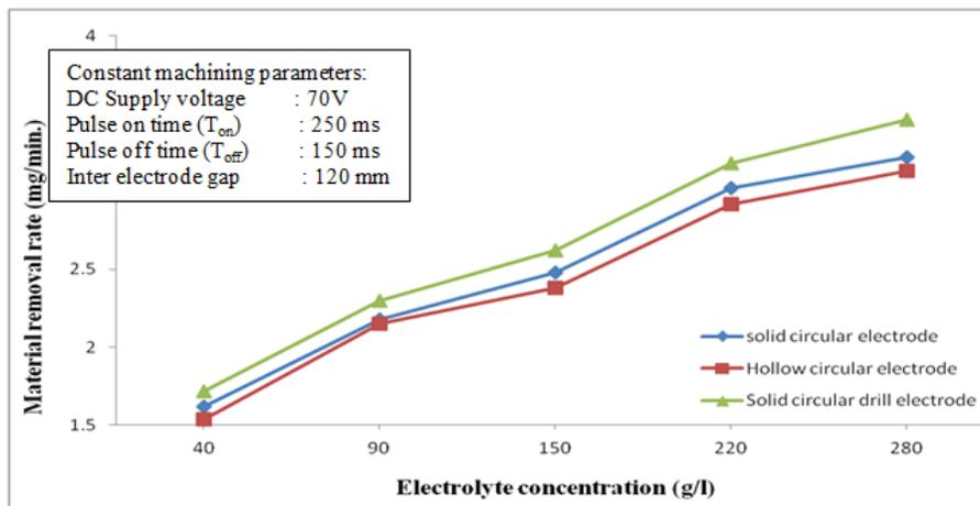
Fig. 4 Variation of MRR with electrolyte concentration for different shapes of electrodes
