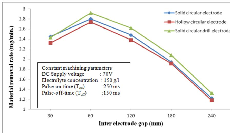
Fig. 6 Variation of MRR with inter electrode gap for different shapes of electrodes
