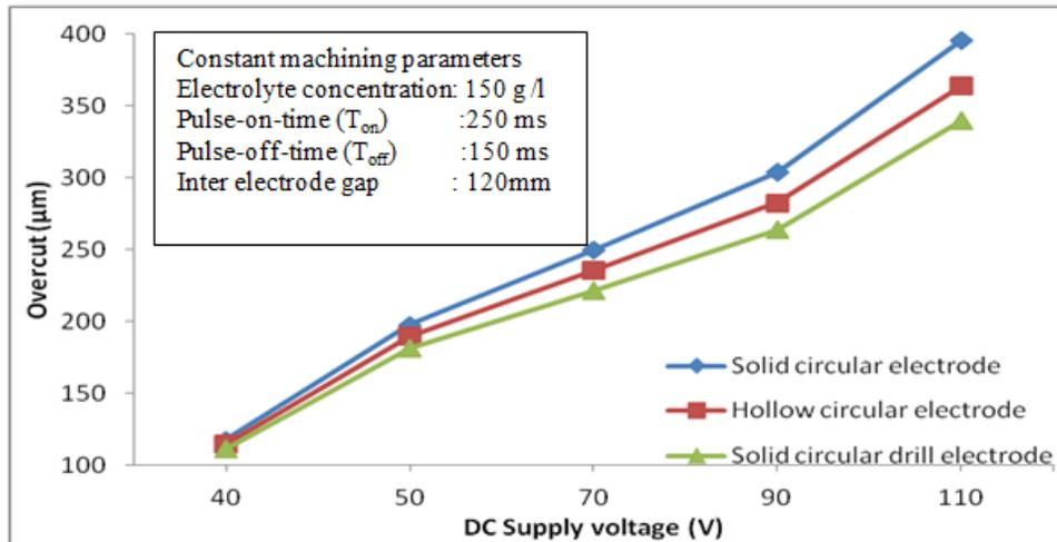
Fig. 7 Variation of overcut with DC supply voltage for different shapes of electrodes
