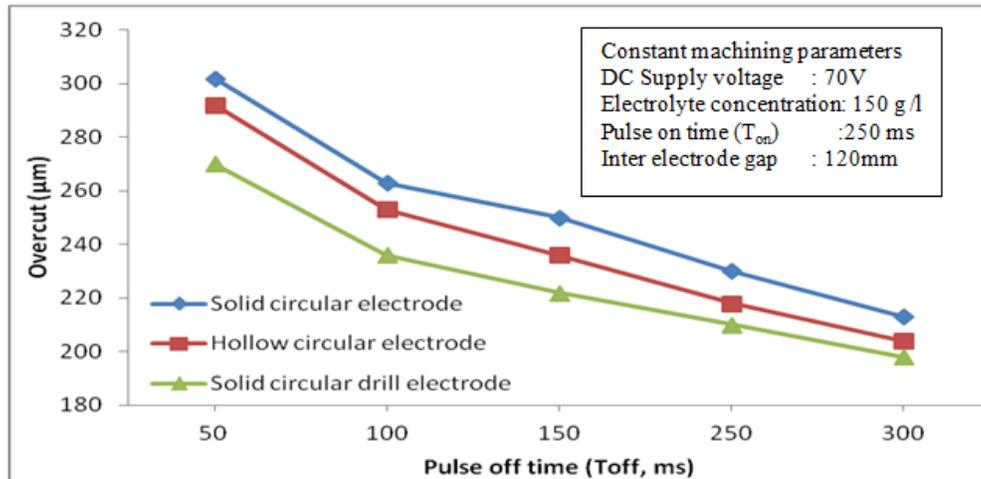
Fig. 9 Variation of overcut with pulse-off time (T<sub>off</sub>) for different shapes of electrode
