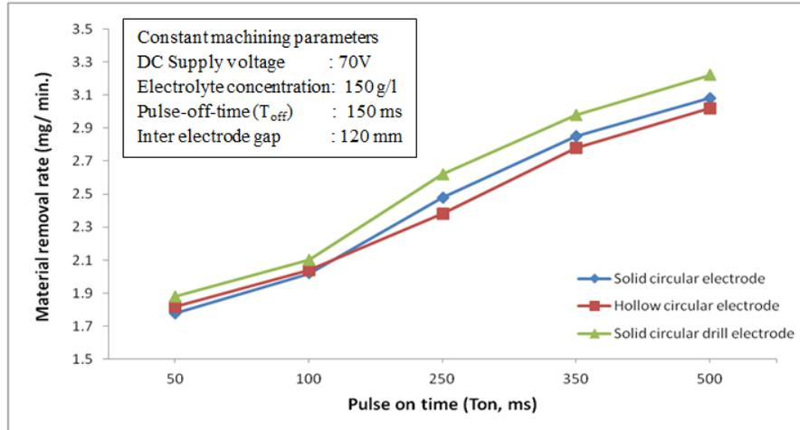
Fig. 5 Variation of MRR with pulse-on-time ( $T_{on}$ , ms) for different shapes of electrodes
