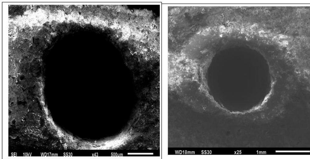
Fig. 5.10 SEM images of machined hole at 70V with (a) solid circular electrode (b) solid circular drill electrode.
