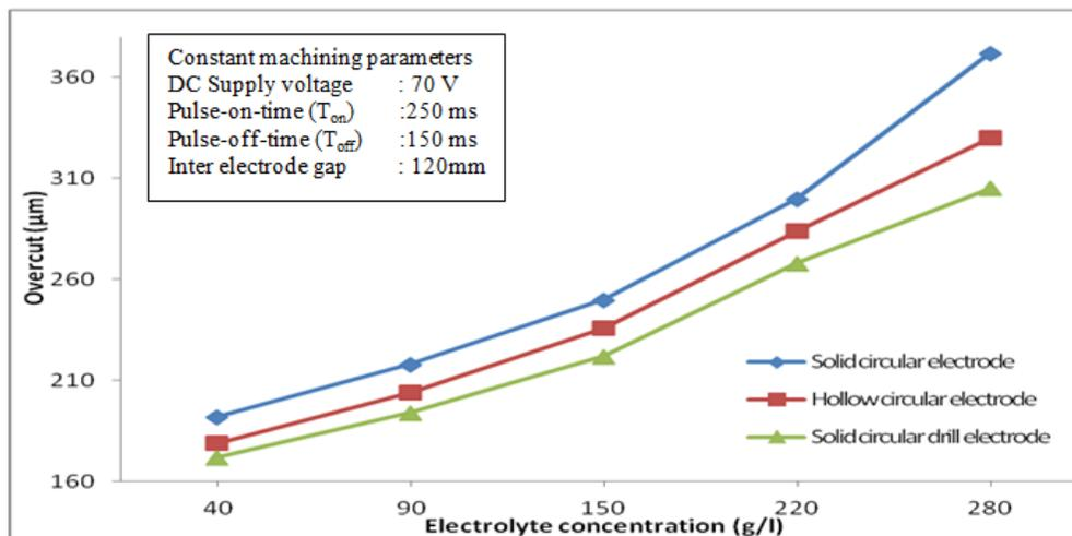
Fig. 8 Variation of overcut with electrolyte concentration for different shapes of electrodes
