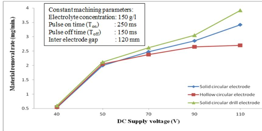
Fig. 3 Variation of MRR with DC supply voltage for different shapes of electrodes
