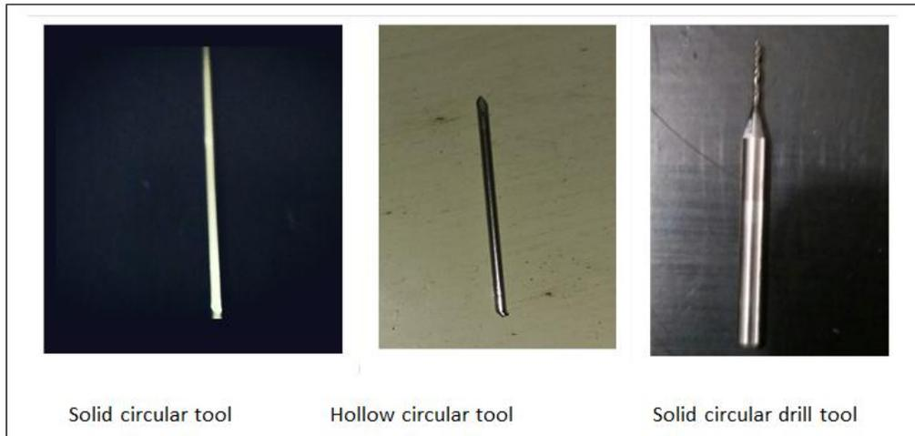
Fig. 1 Different shapes of tool i.e. electrodes used
