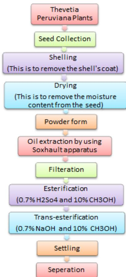
Fig 4. Flow chart of TPSO Extraction Process
