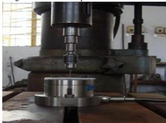
Figure 2.3 Drill Machine, Bit & Dynamometer
