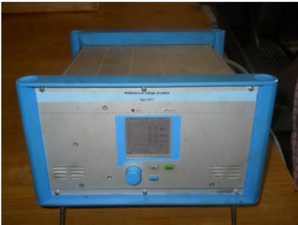
Figure 2.2 Multichannel charge amplifier
