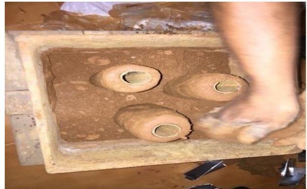
Figure 2. Mould and mould cavity to make the composite bars
