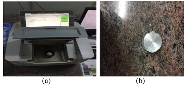
Figure 5. (a) XRF machine (b) Specimen of sample 1
