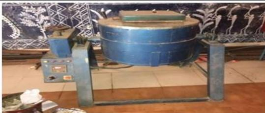
Figure 1. Electric arc furnace for melting of various constituents of the composite
