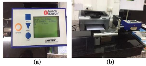
Figure 7. (a) TAYLOR HOBSON roughness checker machine (b) setup for checking roughness
