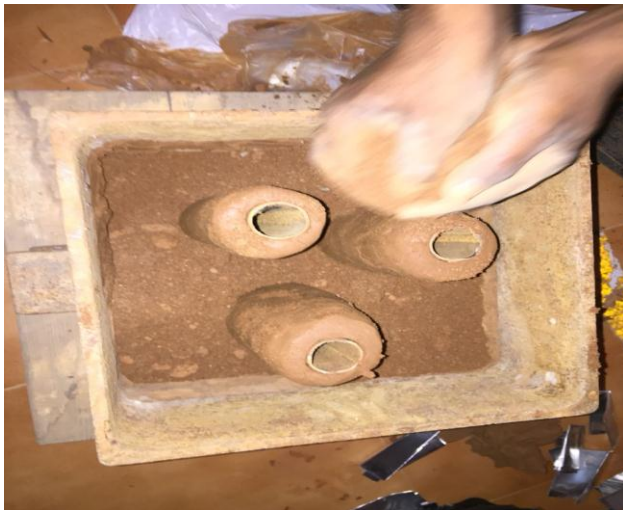
Figure 2.2. Patterns for Producing Mould Cavities
