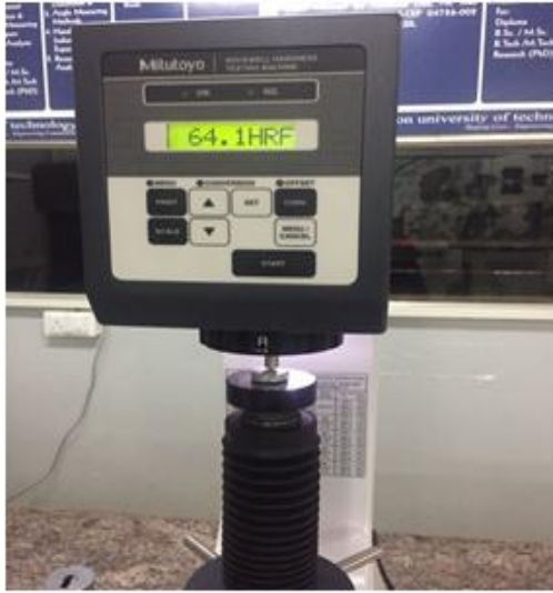
Figure 3.3 Hardness of specimen 2 Rockwell Hardness Testing Machine
