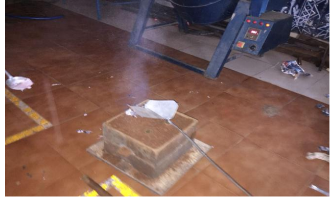
Figure 2.3. Pouring of Molten Metal Into The Mould Cavity
