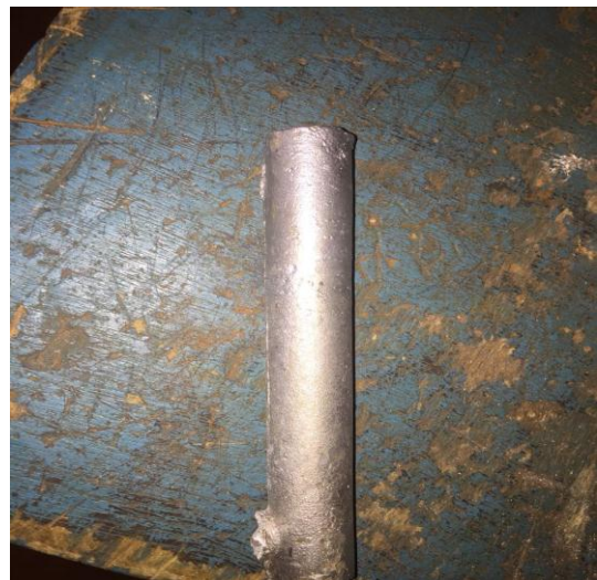
Figure 2.4. Final Product Of Composite Bar of Sand Casting Process
