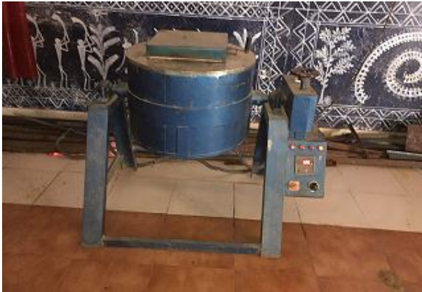
Figure 2.1. Electric Arc Furnace For Preparation Of Molten Metal
