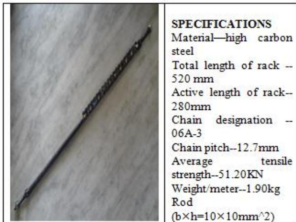
Fig: 2.1 Rack and Pinion Mechanism and its Specifications
