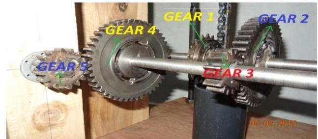
Fig: 4.1 Gear train from rack to generator
