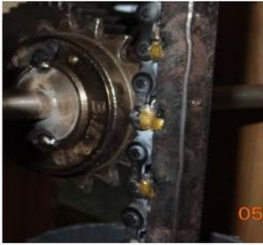
**Fig: 3.1 Rack rod and freewheel alignment**
