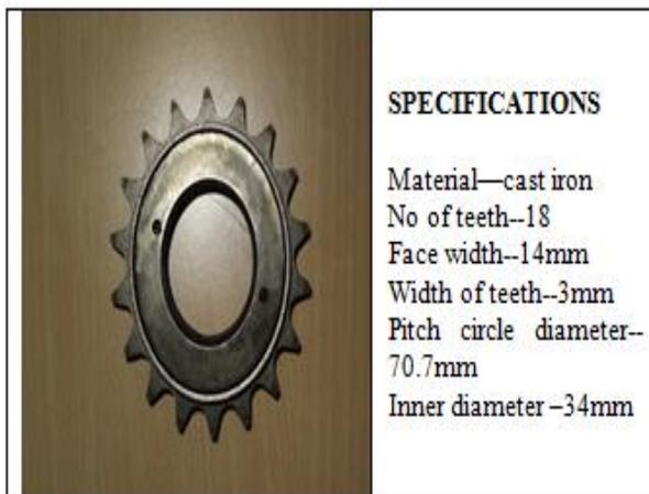
Fig: 2.2 Pinion –Freewheel
