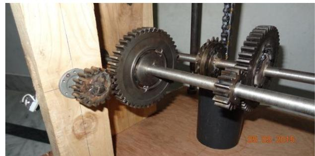
**Fig:3.7 Gear train alignment**
