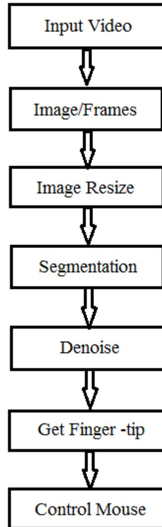
Fig. 1: An overview of our Fingertip recognition and mouse control system
