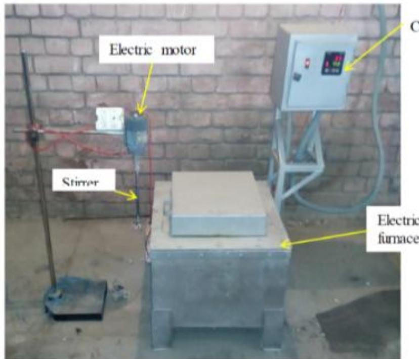
Fig 2 Complete stir casting setup
