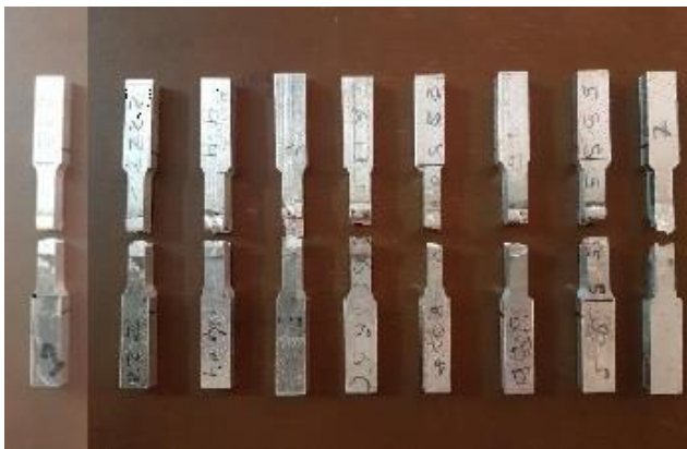
Figure 9. Tensile specimens after tensile testing
