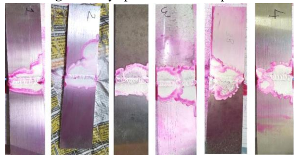
Figure 4. Dye penetrate test samples 1
