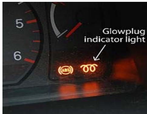
**Figure 4:** Glow plug indicator light in a diesel car [Source: [en.wikipedia.org](http://en.wikipedia.org)[1] ]
