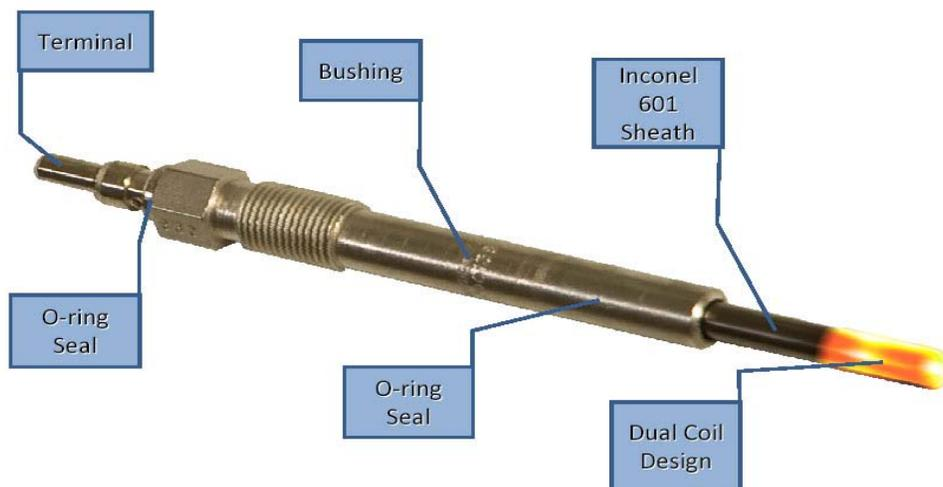
**Figure 2:** Parts of Glow plug [Source: <http://www.dieselryproducts.com>][2]
