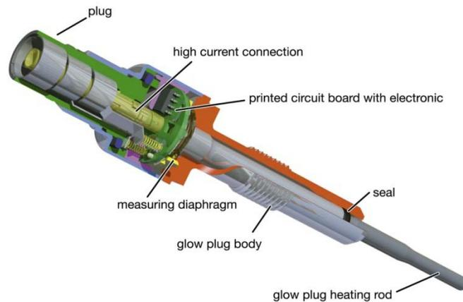
**Figure 3:** Construction of Glow plug [Source: <http://www.motor-car.co.uk> [3] ].
