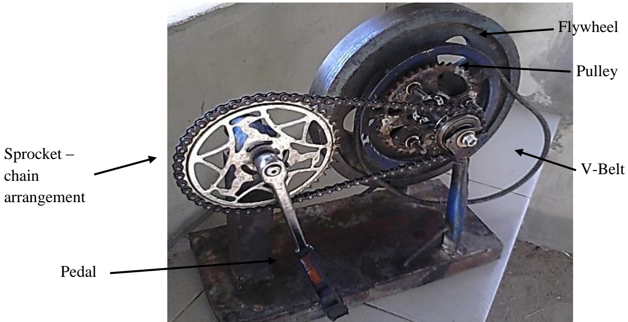
Plate 2: The manual machine that replaces the prime
