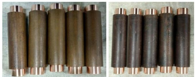
**Fig. 5 Without heat treated Cu electrode and Heat treated CU electrode**
