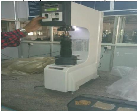
Fig. 6 Hardness testing machine
