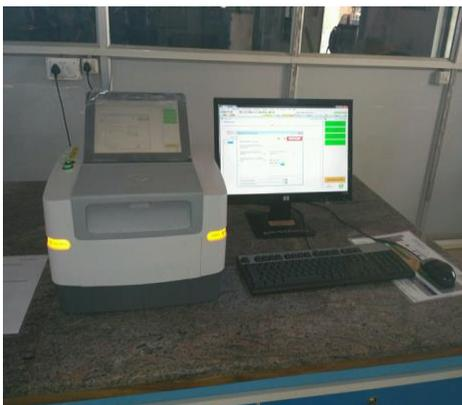
Fig. 7 XRF machining for composition
