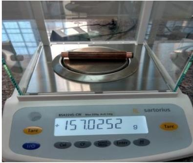
**Fig. 11 Measuring the weight of the tool with the help of Semi Micro Balance**
