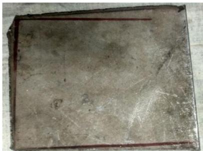
**Fig. 3 INCONEL – 825 Workpiece (Before machining)**
