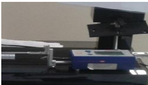
Shows the Talysurf surface roughness testing device for measurement of surface roughness(Ra)
