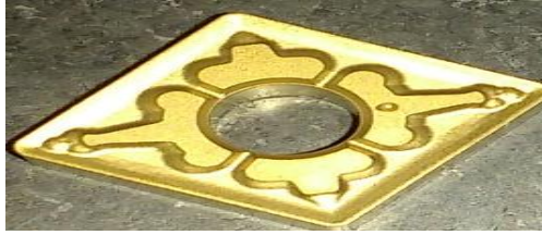
Cutting tool (carbide tipped tool CNMG120408TM-T9125)
