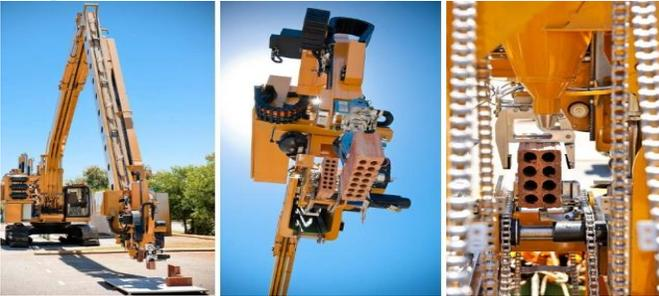
The robot is 92ft (28 metres) long which is connected to its main body. This robot work that can grab bricks, pick them up, and place them down in sequence. 3D computer-aided design (CAD) is used to design house and structure required and robot calculate where each brick should placed. Mortar is also placed on brick by used of human hand. There should leave some spaces for wiring and plumbing.
