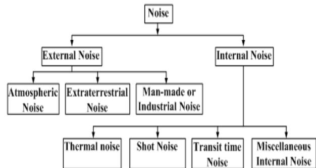
External noise cannot be reduced except by changing the location of the receiver or the entire system. Internal noise on the other hand can be easily evaluated mathematically and can be reduced to a great extent by proper design. As already said, because of the fact that internal noise can be reduced to a great extent, study of noise characteristics is a very important part of the communication engineering.
