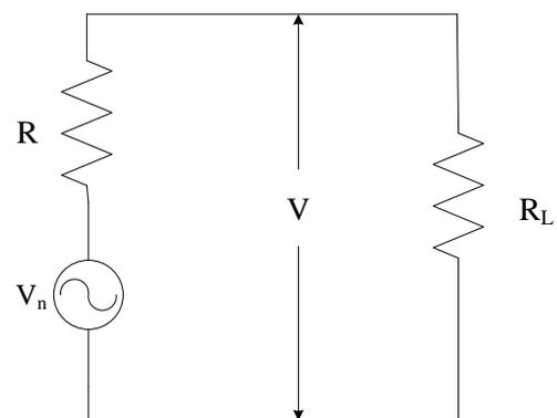
Figure 01: Resistance noise generator
