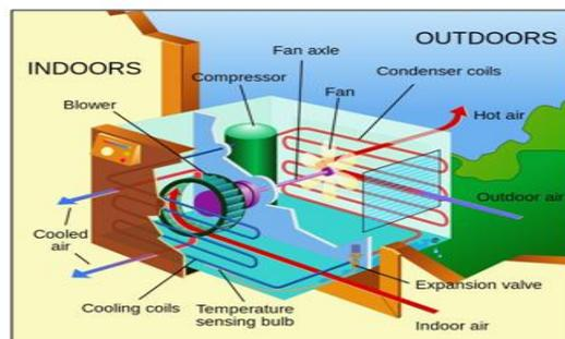
This warm air is drawn in through a grille at the base of the indoor unit, which then flows over some pipes through which the refrigerant (i.e., a coolant fluid) is flowing. The refrigerant liquid absorbs the heat and becomes a hot gas itself. This is how heat is removed from the air that falls on the evaporator coils. Note that the evaporator coil not only absorbs heat, but also wrings out
