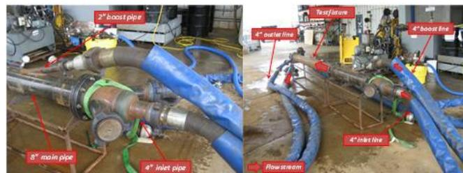
Figure 3: Overview of test setup and details of test fixture. Injector pipe (left) and full piping system (right)
