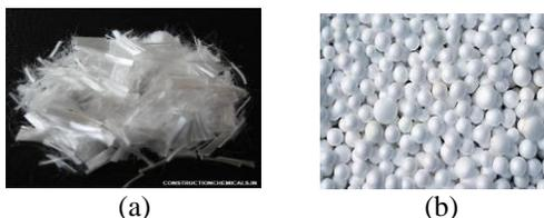
**Figure 1:** (a) Polypropylene fiber (b) EPS beads
