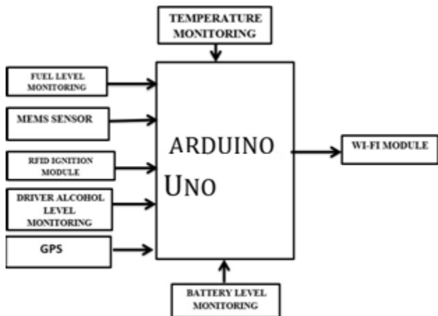
Figure 1: Functional pattern of automobile monitoring system
