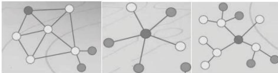
**Figure 3:** Mesh topologies (left), star (centre) and star cluster (right).
