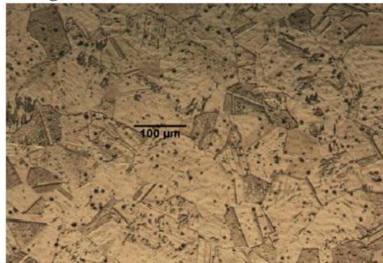
**Figure 5:** Different zone microstructures in resistance spot welding
