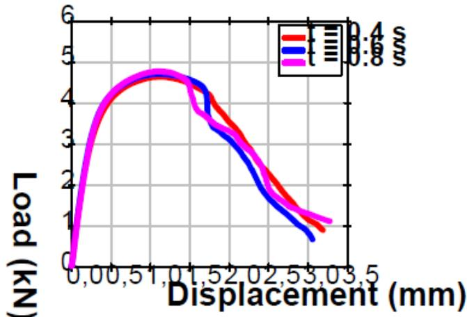
Figure 8: Weld time effect on tensile test of welded joint: AISI 403, I = 8 kA, e = 0.8 mm
