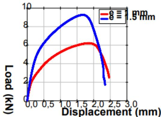
Figure 7: Influence of sheet thickness on welded joint tensile test: AISI 304, I = 6 kA, t = 0.6 s
