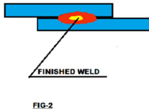
Copper electrode conducts an electric current through the workpieces to generate heat. The amount of heat produced is determined by the resistance of the workpieces, the thermal conductivity of the metal, and the length of time that the current is applied. We computed how much heat will be generated using joule's equation of heating.
