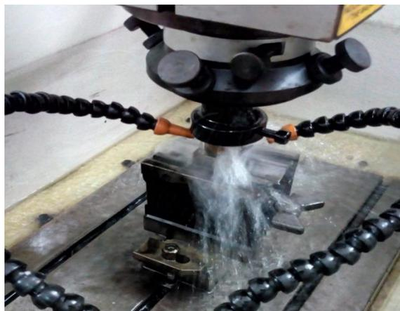
Figure 3: Flushing Method
