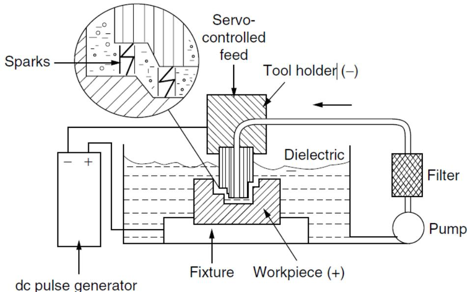
Figure 2: Schemetic Diagram of EDM
