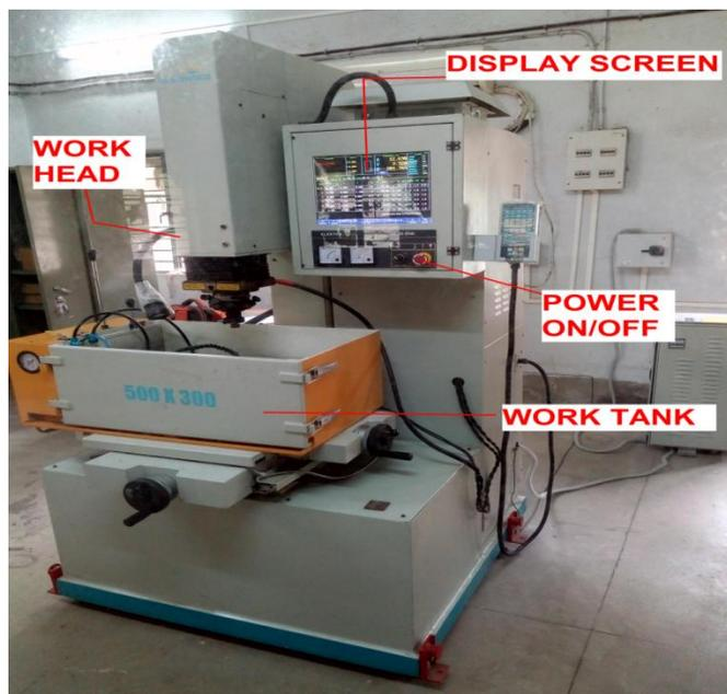
Figure 4: Set up of Electric discharge machining
