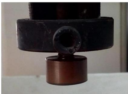
**Figure 6:** Tool holder with Workpiece and tool
