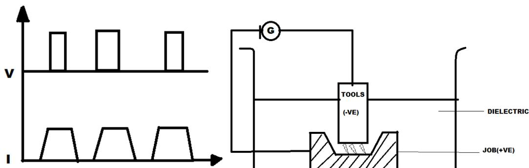
Figure 1: Working principle of EDM process
