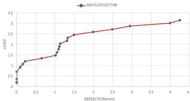
Figure 7: Load vs. deflection at Midspan
