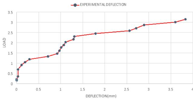
Figure 6: Load vs. deflection at midspan
