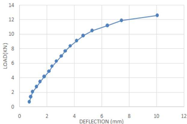
Figure 6: Load vs. deflection at midspan for 50-50-200-1.2-1200
