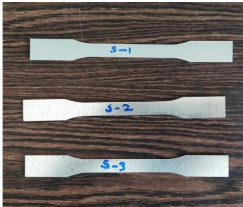
**Figure 1:** Samples of coupon
