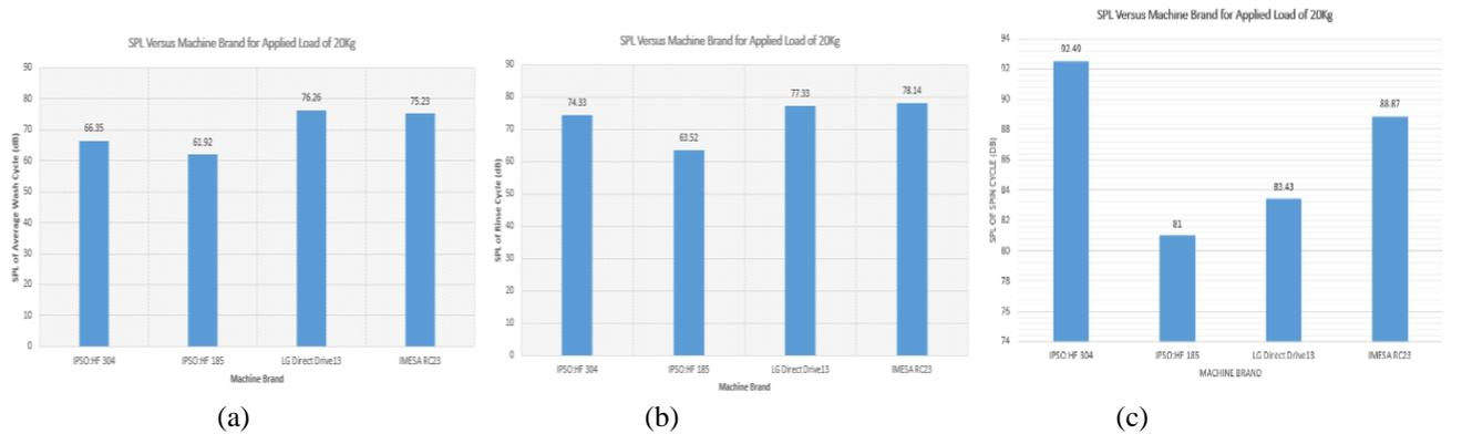
Fig. 5 (a-c): Plot of SPL against machine brand for the three cyclic mode with an applied load of 20kg
