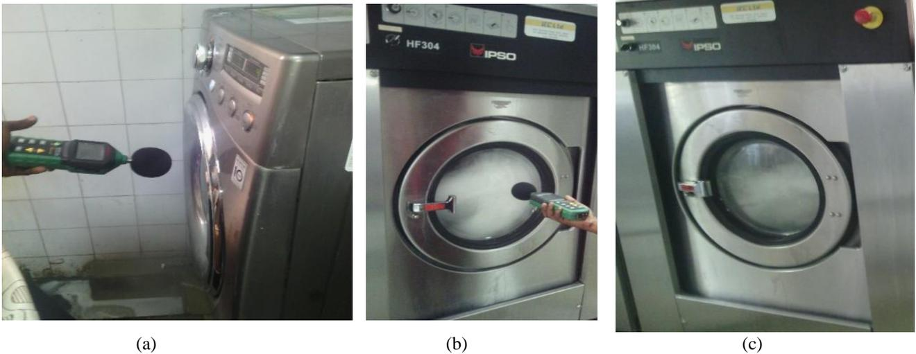
Fig.3: Measurement of overall noise power level with SLM at different (a) washing (b) rinsing and (c) spinning positions of the machines.
