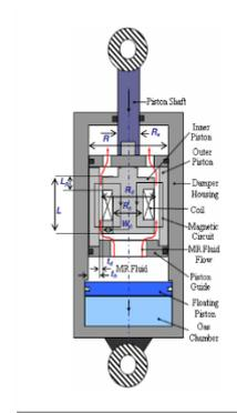
Fig. 1: (a) 3D Schematic of the Prototype Washing machine (b) Schematic configuration of the MR damper.
