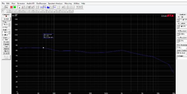
Fig. 7c: Calibration of SLM measurement for the spin cycle of LG Direct Drive 13 at SPL of 81.28dB with applied load of 30 kg
