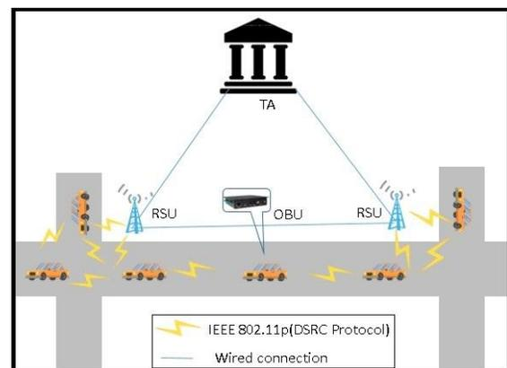
Figure 1: The architecture of VANETs
