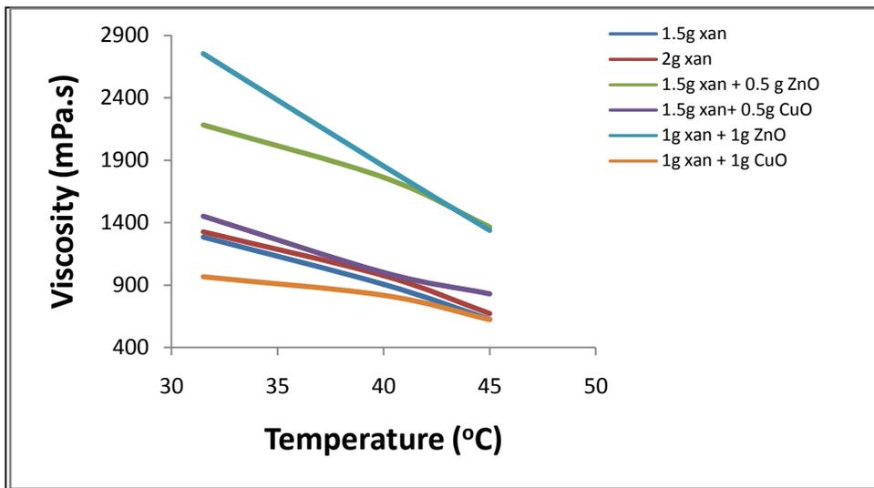
Figure 1: Viscosity against temperature at 60 rpm for drilling fluid containing bentonite, xanthan and nanoparticle in different proportion
