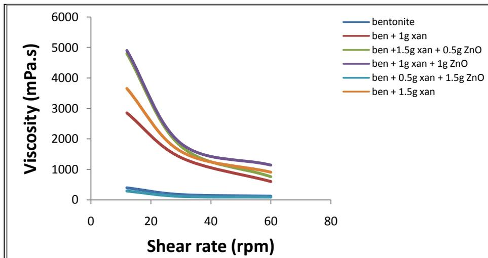
Figure 2: Viscosity against shear rate of drilling fluid for different concentration of xanthan gum and ZnO nanoparticle at 40°C
