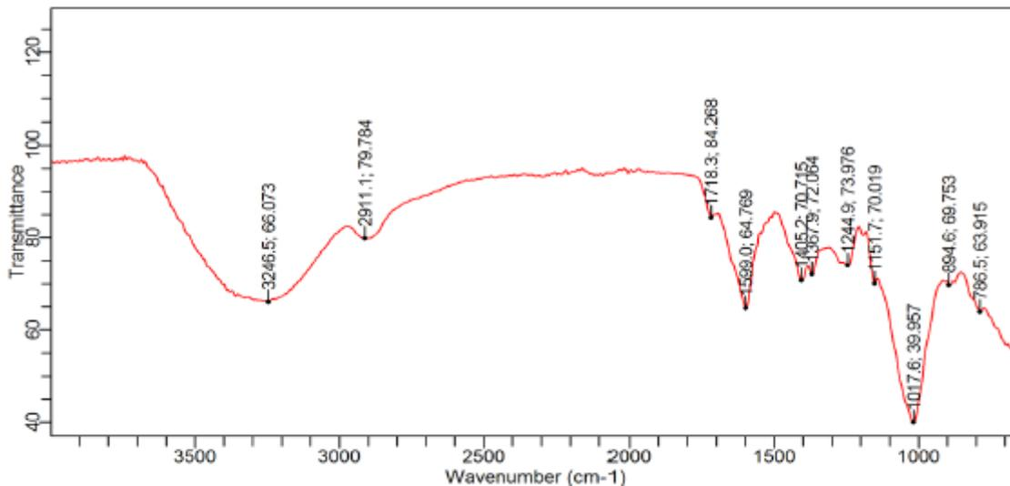
Figure 5: Spectrum of blend of CuO nanoparticles and xanthan gum in equal proportion
