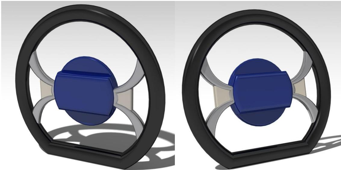
**Figure 5:** Unique Steering wheel with array of grip sensor designed with CATIA
