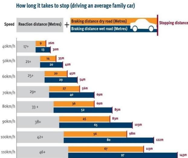
Figure 1: Overall Stopping Distance of vehicle at various speeds
