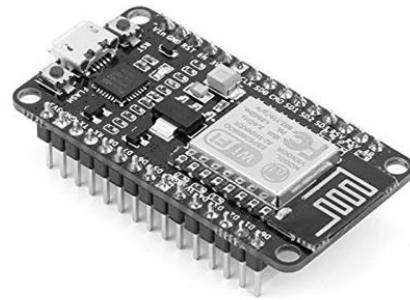
**Figure 2:** ESP8266 Wi-Fi Module
