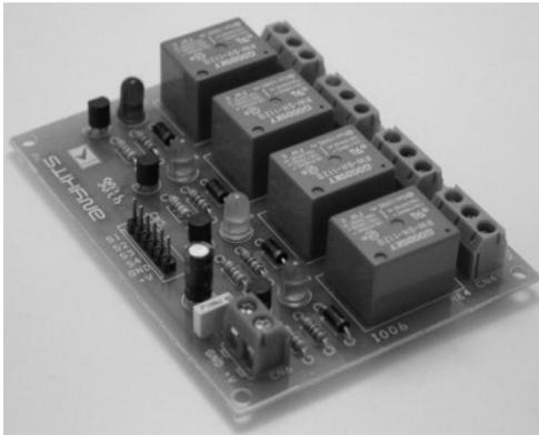
Figure 4: Relay Board
