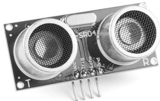
**Figure 3:** Ultrasonic Sensor
