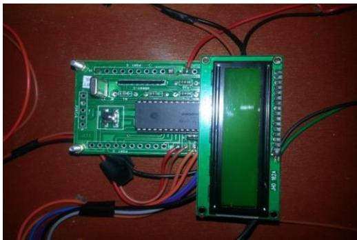
**Figure 1:** PIC16f877 with LCD
