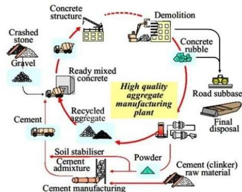
Figure 8: Concrete recycling process
