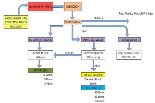
Figure 9: Recycling process
