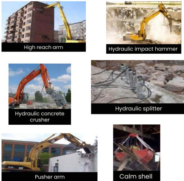
Figure 7: Types of demolition equipment
