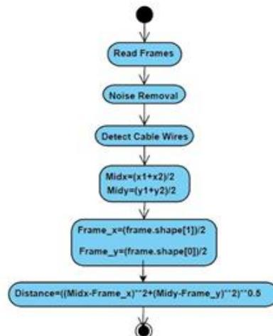
Figure 8: Activity Diagram for measuring Stagger
