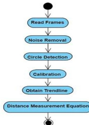
Figure 5: Activity Diagram for measuring Implantation
