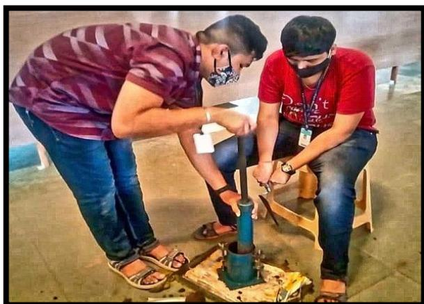
Figure 3: Performing Standard proctor test
