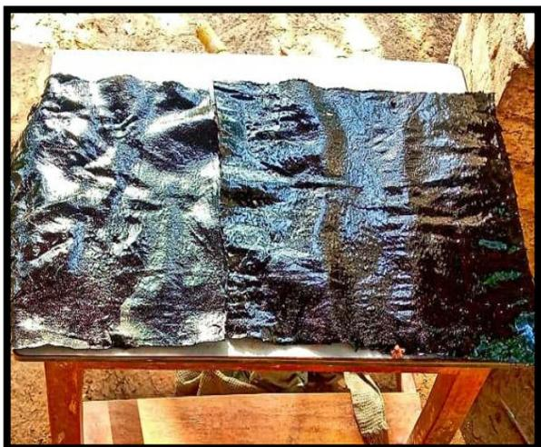
Figure 2: Cotton cloth coated with bitumen
