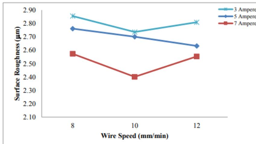
Surface roughness is impacted by wire speed, as shown in Fig. 3, where the lower the wire speed, the rougher the surface roughness value. Similarly, increasing wire speed will make the surface roughness value smoother, but increasing wire speed will make the workpiece surface rough again. It was discovered that by adjusting the machine parameters to a low pulsed current and a short pulse-on period, an outstanding machined finish may be achieved. This is due to the fact that as the
