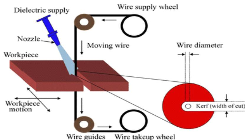
A dielectric, or deionized water, is used in the wire-cutting process. Deionization produces pure water that can be used as an insulator. Furthermore, because the fixed water contains minerals, the wire is extremely conductive. Meanwhile, the operation of water circulation on the wire cut system was carried out to set the conductivity of water. Figure 1 depicts a diagram of the wire-cutting process.
