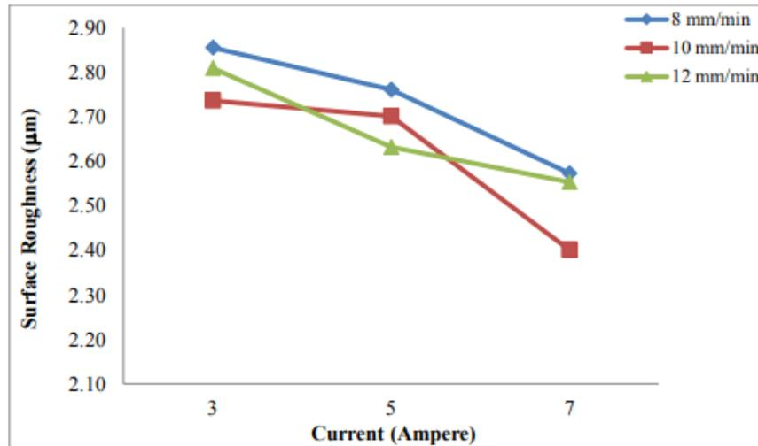
Surface roughness is highly impacted by currents, as shown in Fig. 2. It is obvious that when the current value is higher, the surface roughness tends to be
