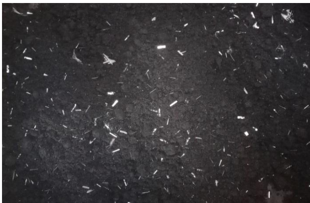
Figure 2: Mixing of SCBA, BF Slag and glass fibre
